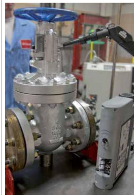
Low emissions OEM packing testing
