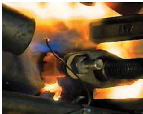
Low emission packing passes fire testing
